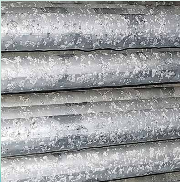
White Rusted Coil without Pass-Protect
